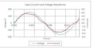
Input AC Current Waveform (ITHD = 7.3%, 50% Load)
