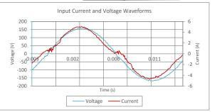
Input AC Current Waveform (ITHD = 13.2%, 50% Load)
