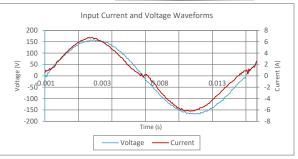
Input AC Current Waveform (ITHD = 10.39%, 50% Load)
