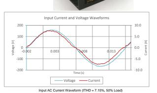
Note: All measurements were taken with input voltage at 115 V nominal at 60 Hz.
