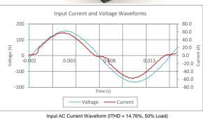
Note: All measurements were taken with input voltage at 115 V nominal at 60 Hz.
