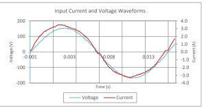
Input AC Current Waveform (ITHD = 5.67%, 50% Load)
