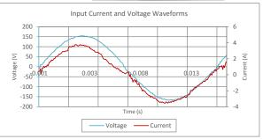
Input AC Current Waveform (ITHD = 7.053%, 50% Load)
