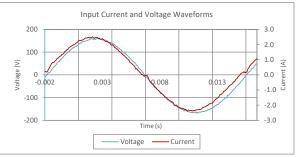
Input AC Current Waveform (ITHD = 6.69%, 50% Load)
