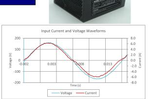
Input AC Current Waveform (ITHD = 7.58%, 50% Load)
