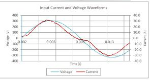
Input AC Current Waveform (ITHD = 19.81%, 50% Load)
