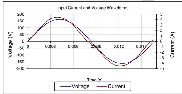
Input AC Current Waveform (ITHD = 7.17%, 50% Load)
