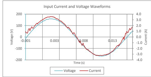
Input AC Current Waveform (ITHD = 3.95%, 50% Load)
