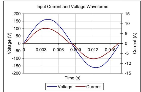
Input AC Current Waveform (ITHD = 12.14%, 50% Load)
