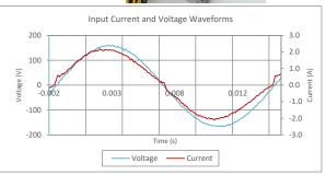
Input AC Current Waveform (ITHD = 4.35%, 50% Load)
