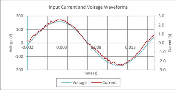
Input AC Current Waveform (ITHD = 6.26%, 50% Load)
