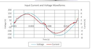
Input AC Current Waveform (ITHD = 10.383%, 50% Load)
