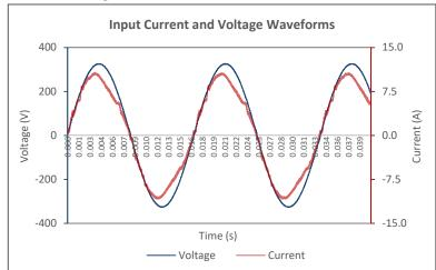
Input AC Current Waveform (ITHD = 7.48%, 50% Load)
