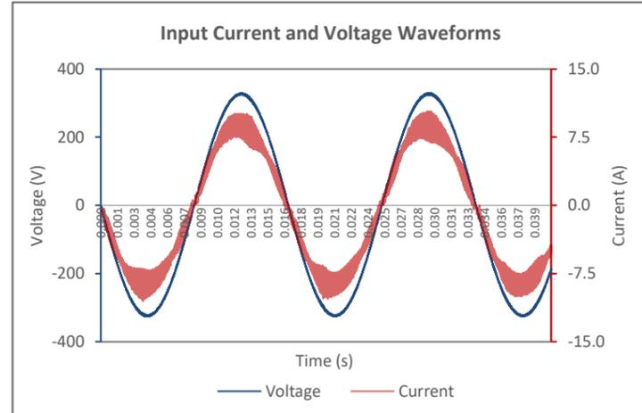
Input AC Current Waveform (ITHD = 2.47%, 50% Load)
