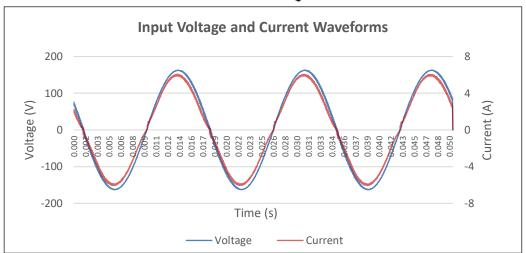
Input AC Current Waveform (ITHD = 4.22%, 50% Load)
