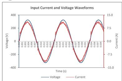
Input AC Current Waveform (ITHD = 5.93%, 50% Load)
