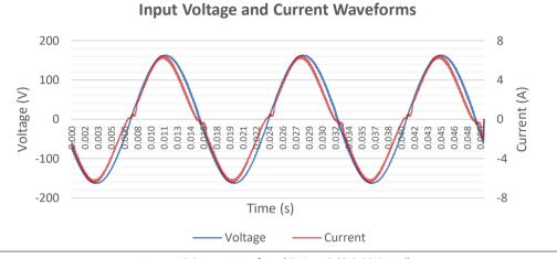
Input AC Current Waveform (ITHD = 10.69%, 50% Load)
