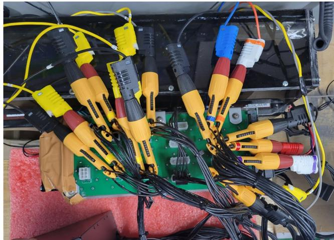
Figure 3: Insulated Piercing Probe to Measure the Multi-Output Voltages of Desktop Power Supply
