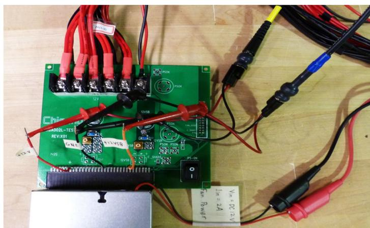
Figure 4: Sense Line, when provided, is used to measure the output voltages
