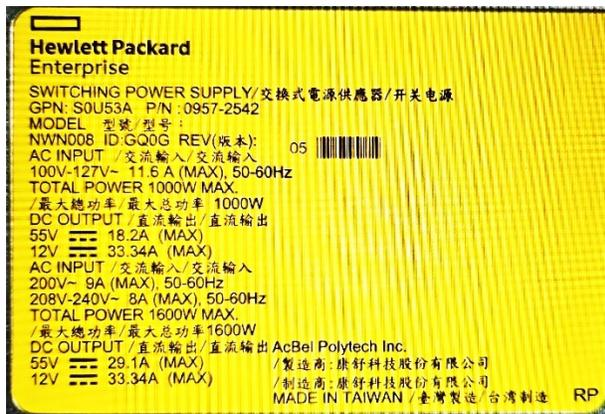
Figure 12: Multi Rail Power Supply Label
