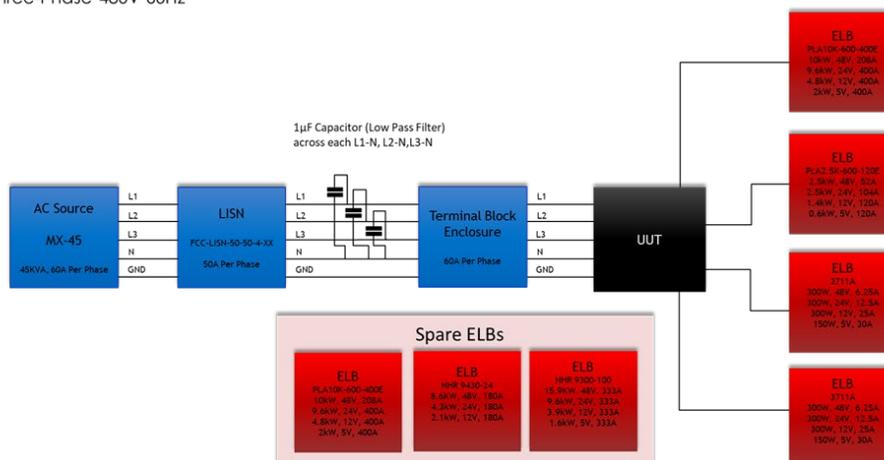
Figure 9: 230V Line Diagram with Load Bank Capabilities
