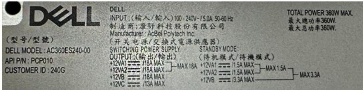
Figure 10: Multi Rail with Sub-Group Current Limits Power Supply Label
