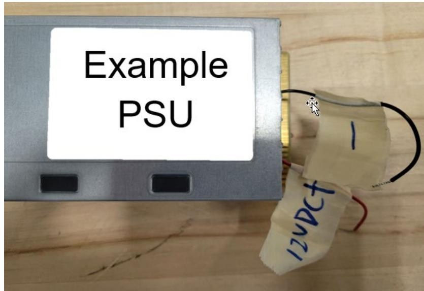
*Figure 8: External Fan Power Labeled*
